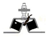
The mount on the left is the type used under 2GM to 4LH series engines, if you need to pass a Cat 4 inspection for off-shore, put a wire or small chain through the centre 'nose' and over the top of the top metal piece and 'Talurite', crimp or u-bolt the ends together. I have never seen this mount fail because the bonding failed from reasonable use. The failures were always incorrect installation, age, or they became covered in diesel.
