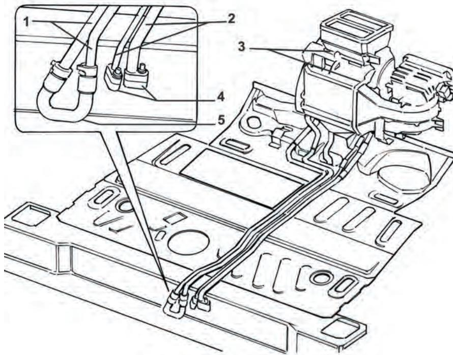
1: engine coolant delivery and return pipes;
