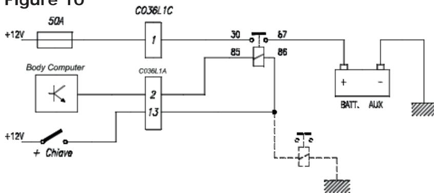
► Ground point nearest to component: choice between A, B, C or pin 2 of connector CO36L1C
