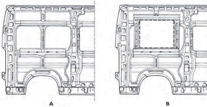
A: Original solution; B: solution with added peripheral frame.
