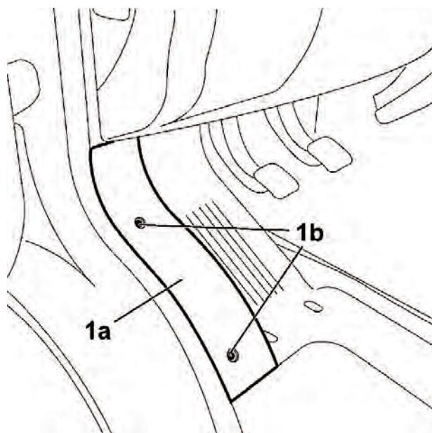
25. Put back in place the B-pillar lower cover (1a) and fix it with screws (1b).
