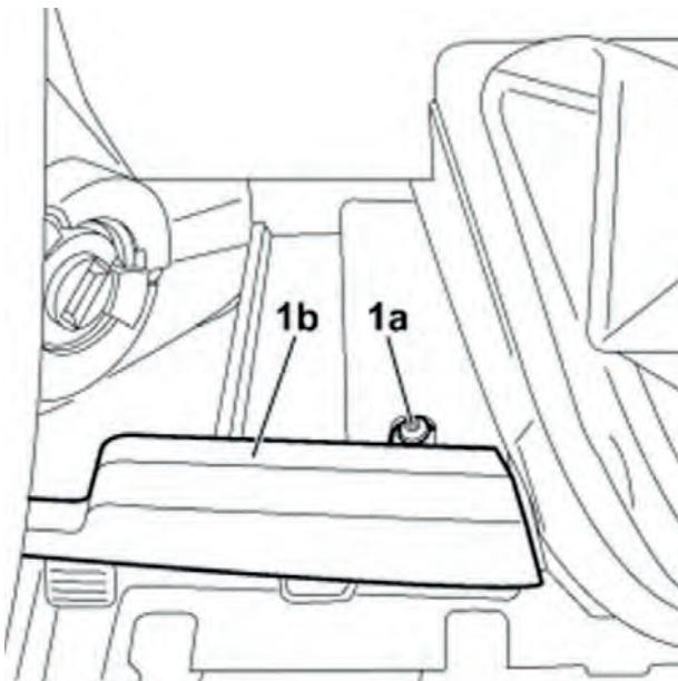
5. Undo the screws (1a) fixing the lower left trim of the dashboard (1b) located to the left of the steering wheel.
