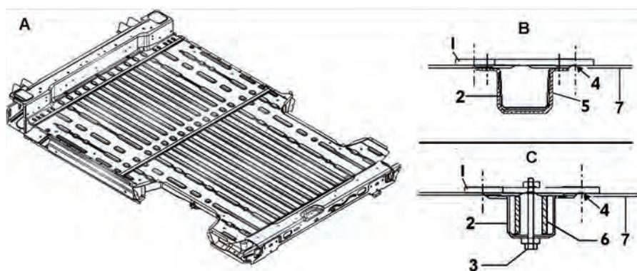
1: Upper plate - 2: Longitudinal - 3: Connection - 4: Anchoring screws
