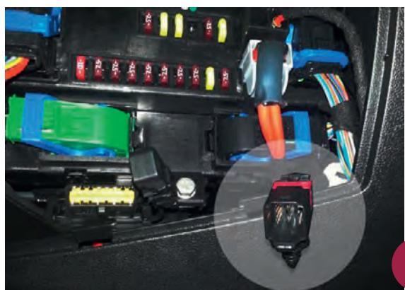
Figure 4 - Connector ready for connecting harness B
