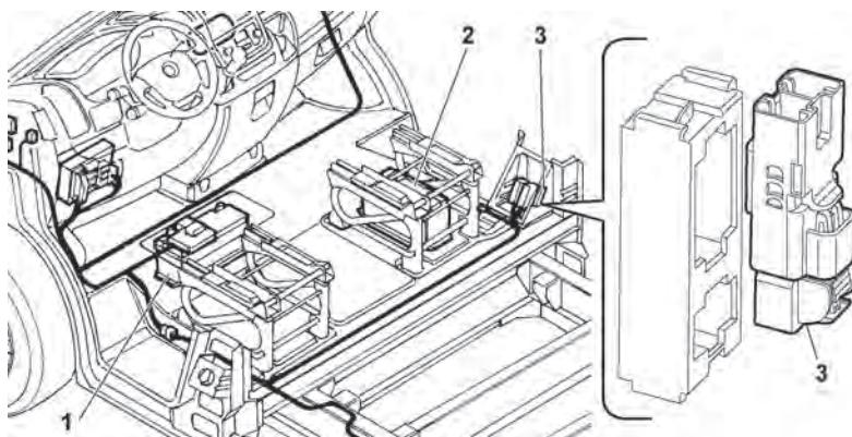
1. Main battery – 2. Auxiliary battery – 3. Two-way connector
