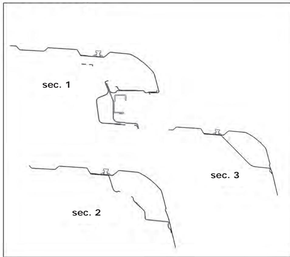
**Roof rack attachment point sections**
