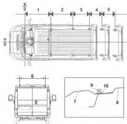
7. Top exterior. – 8. roof – 9. roof rack pin – 10. roof rack attachment reinforcement –
