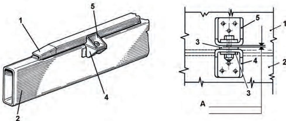
1: Counterframe; 2: Frame; 3: Spacer; A: Gap between the frames: 4-5 mm.
