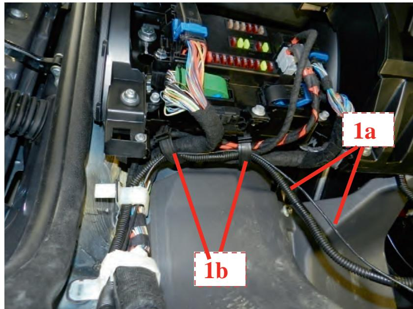
► **NOTE: If the wiring cannot be inserted in the duct and/or retaining clips as previously explained, it should be placed beside the original wiring of the vehicle and secured to it using plastic bands.**
