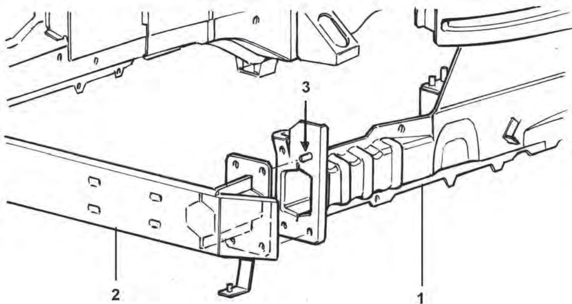
2: front crash box cross-member - 1: controlled impact absorption strut
