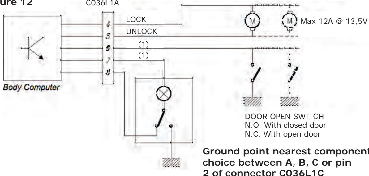
▶ Note (1): In the absence of door open switch (if original Fiat Chrysler Automobiles S.p.A. locks are not used, see chapter 6) pin 6 of connector C036L1A can be left disconnected.
