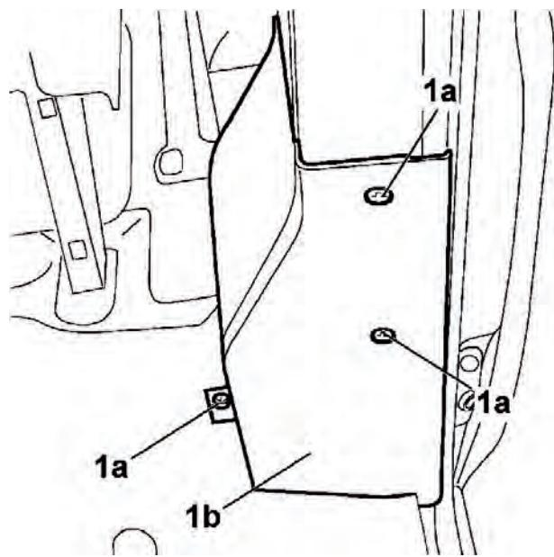
8. Undo the fixing screws (1a) and remove the kick plate connector (1b).
