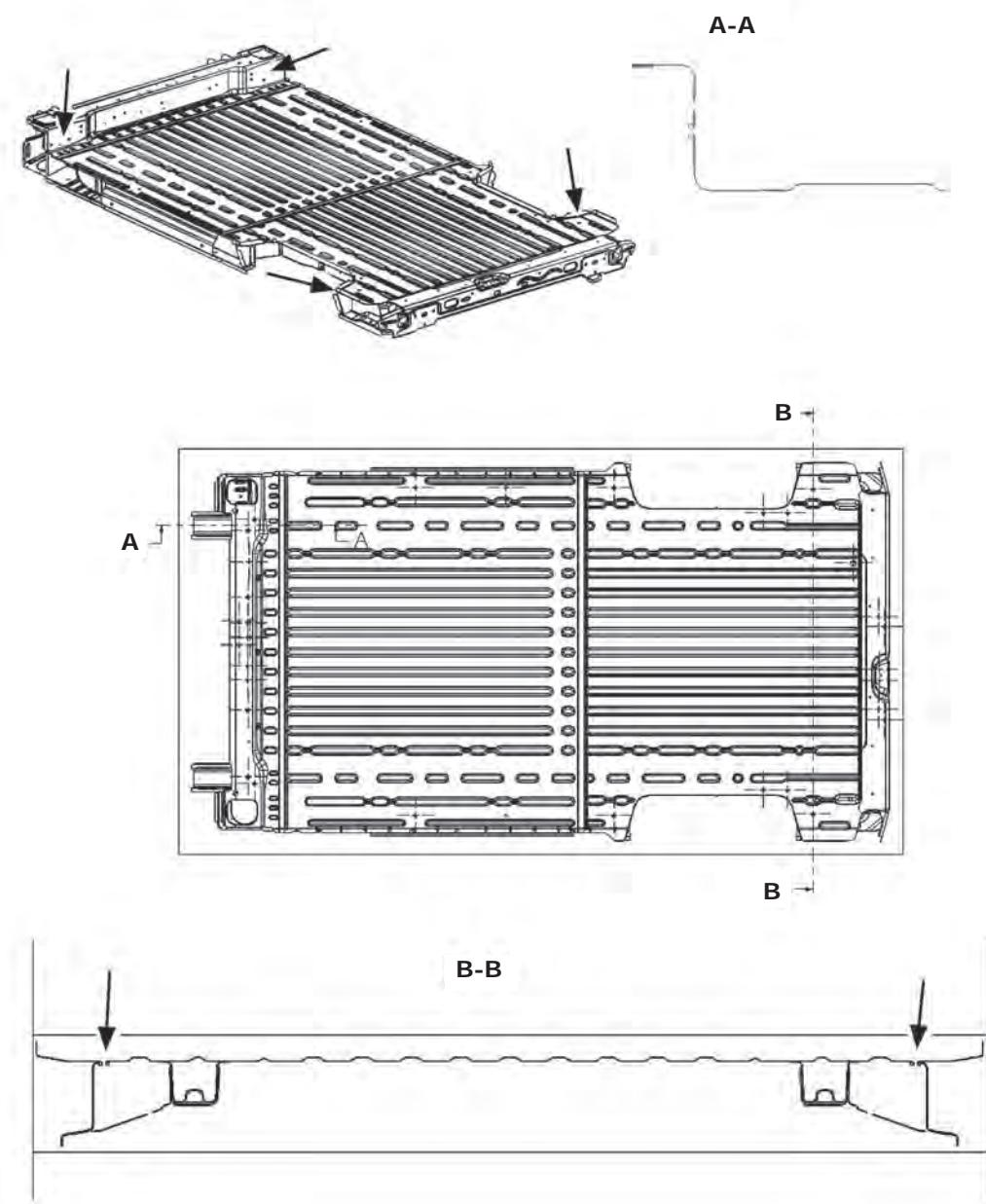
Load retaining hooks on floor
