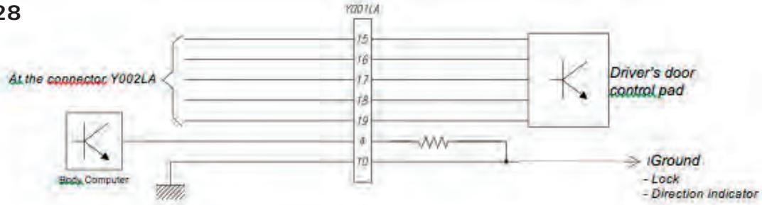
Mirror switch wiring diagram
