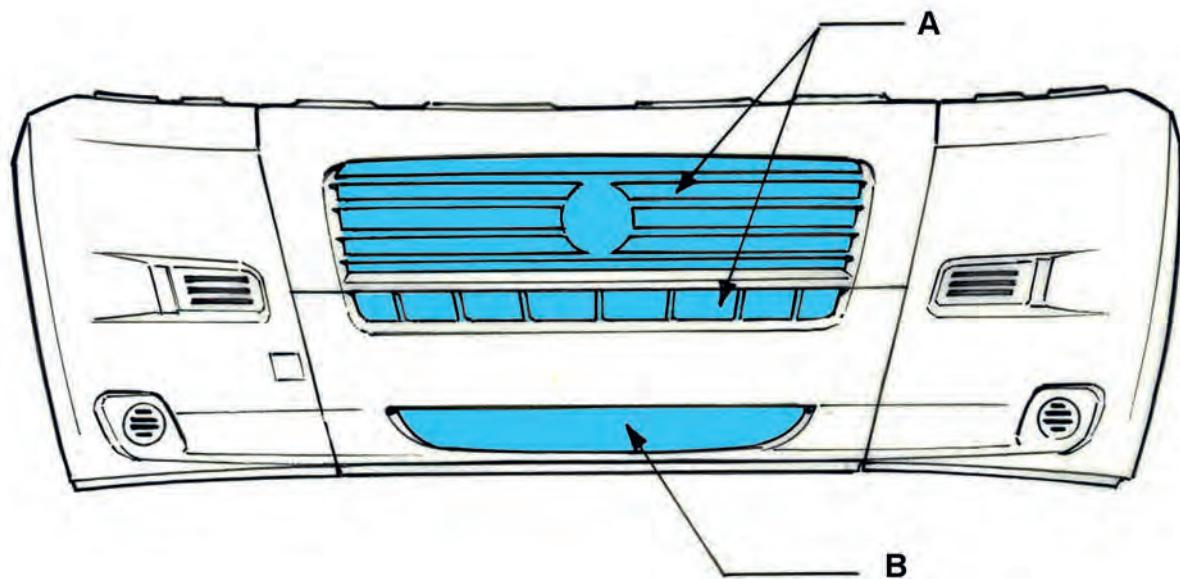
If modifications to the vehicle front are required, the air permeability surface must be uniformly distributed, maintaining the values used on the original version, over the areas corresponding to the radiator (see diagram below).
