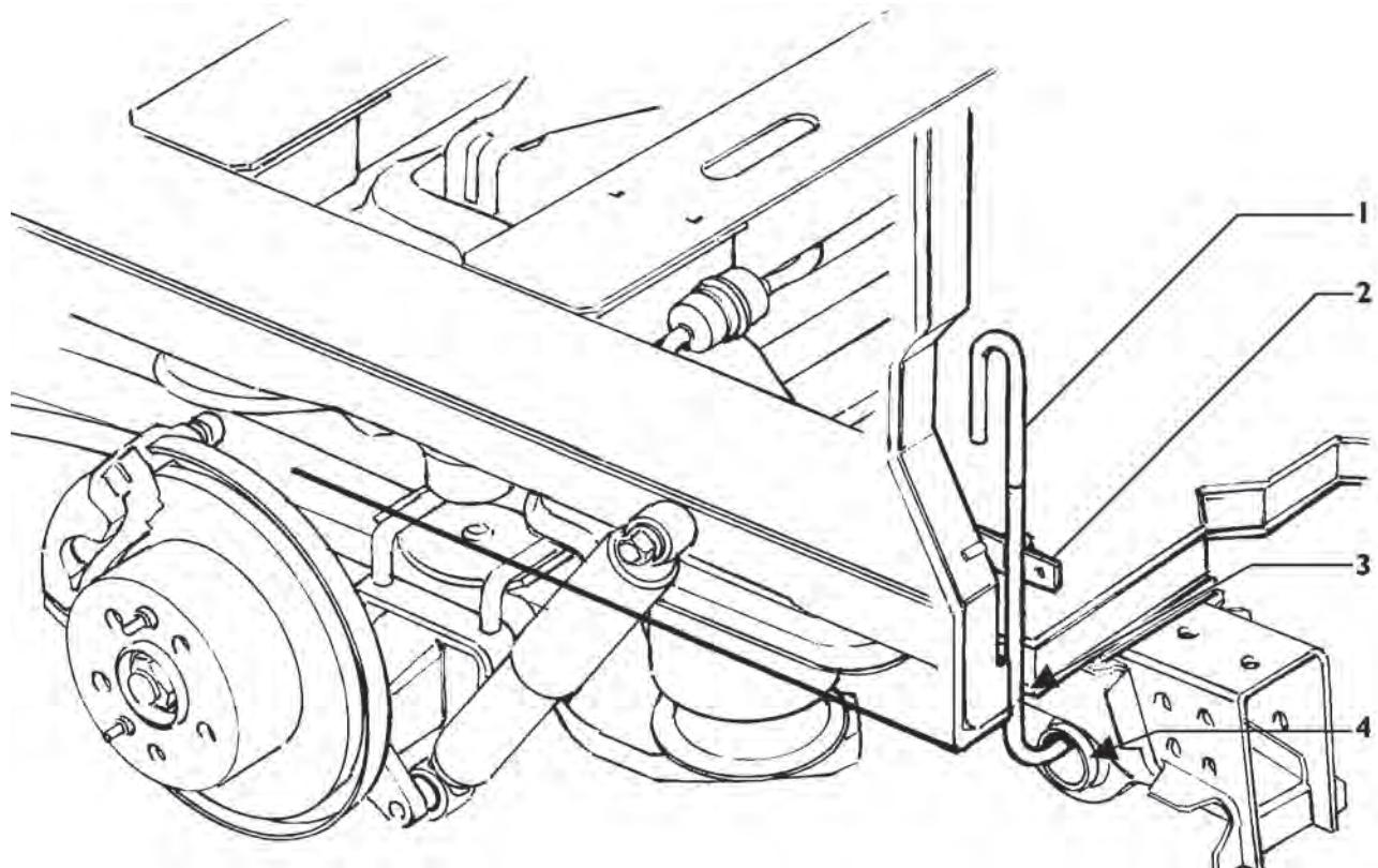
In the figures below you will find the indications on how to fit the rubber pipe.
