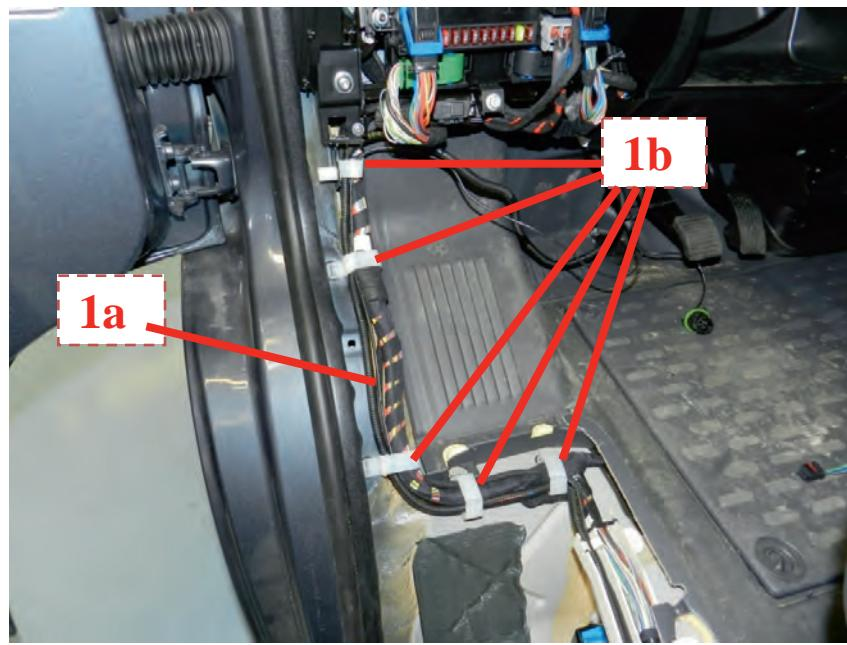
16. Place the wiring (1a) of the control unit inside the retaining clips (1b) of the vehicle wiring.
