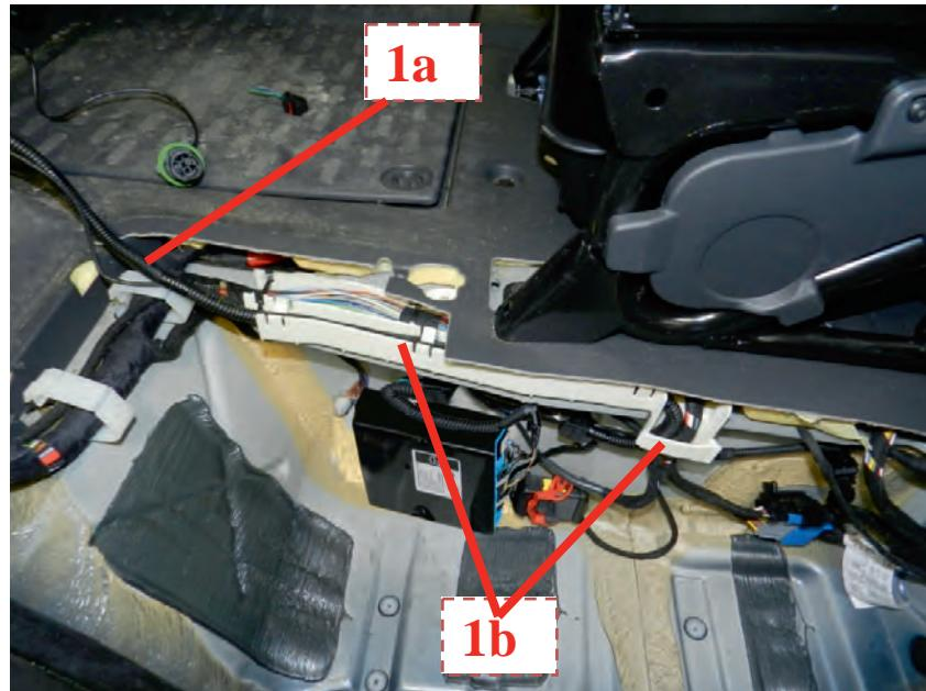
15. Place the wiring (1a) of the control unit inside the retaining clips (1b) of the vehicle wiring.
