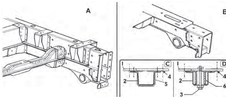
1: upp. plate - 2: longitudinal member - 3: attachment - 4: reinforcing plate
