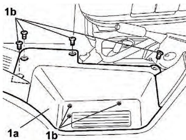
24. Put back in place the sill mould corner part (1a) and fix it with screws (1b).
