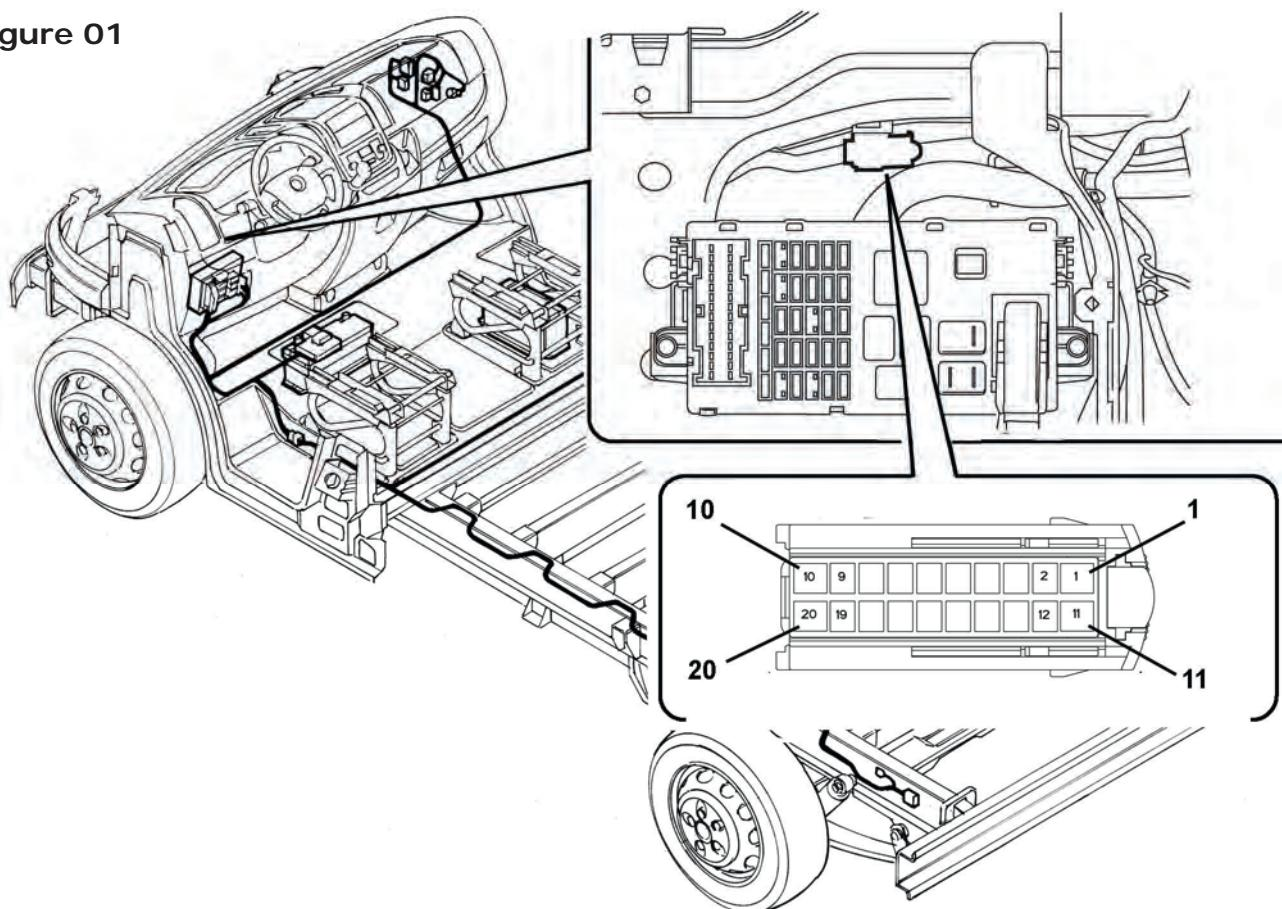
► **NOTE: In the detailed view, the connector is seen from the cable entry side**
