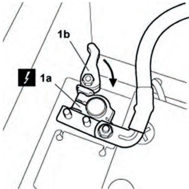
31. Put back in place the cover (1a) and fix with the plugs (1b).
