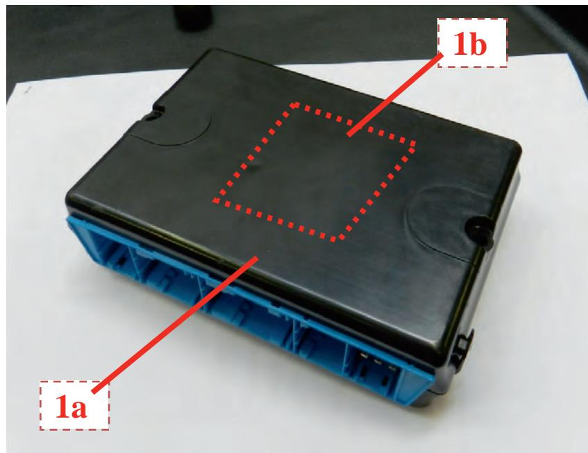
12. Thoroughly grease the surface of the body where the control unit will be positioned with heptane (or isopropyl alcohol). Remove the protective film of the adhesive surface from the Velcro, then position the control unit on the vehicle as shown in the figure, making sure it is firmly secured.
