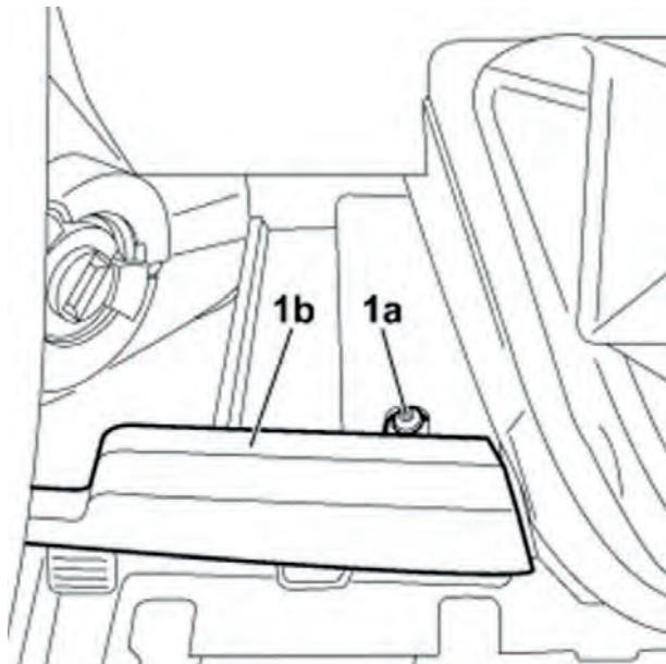
29. Put back in place the fuse-box cover (1) and fix it with the screws (2).
