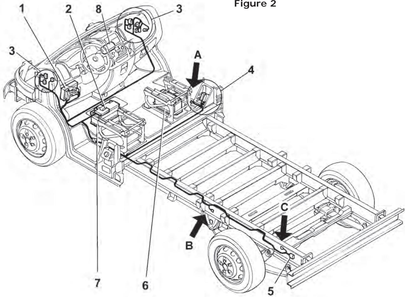
1. Dashboard fuse control unit – 2. Battery fuse box – 3. Connector group for doors and aerials – 4. Side fuse/relay box with 16, 15 and 2-way connectors for coach-builder interfaces – 5. Rear services connector – 6. Possible location of auxiliary battery
