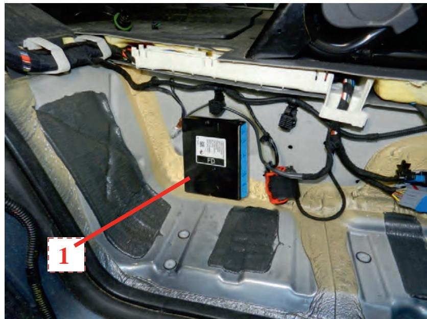
13. Take the wiring supplied in the kit and connect the electrical connections (1a) to the control unit, then use the bands (1b) on the vehicle to secure the control unit wiring and that of the vehicle previously unfastened.
