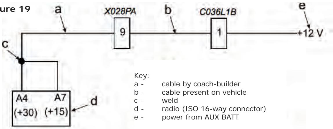
Terminal for hole 9 of connector X028PA: Tyco p/n 282375-1 (cable 1.5 mm<sup>2</sup>)
