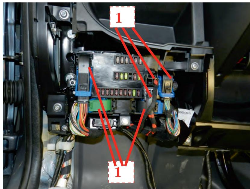
18. Undo the screws (1a) and the nut (1b) securing the Body Computer.
