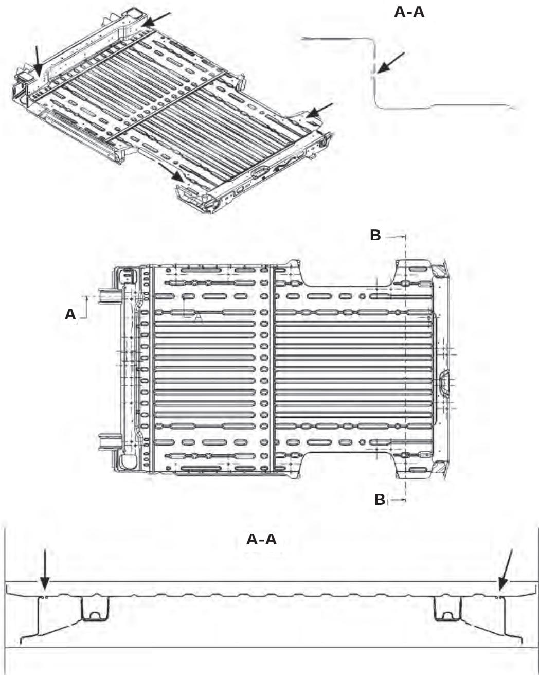
**Load retaining hooks on floor****Medium wheelbase**
