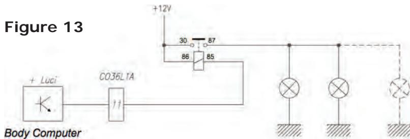
Ground point nearest to component: choice between A, B, C or pin 2 of connector C036L1C
