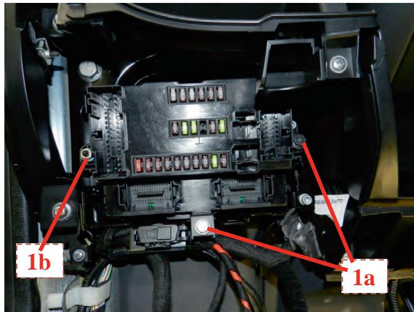
19. Remove the Body Computer being careful not to damage the wiring-harness.
