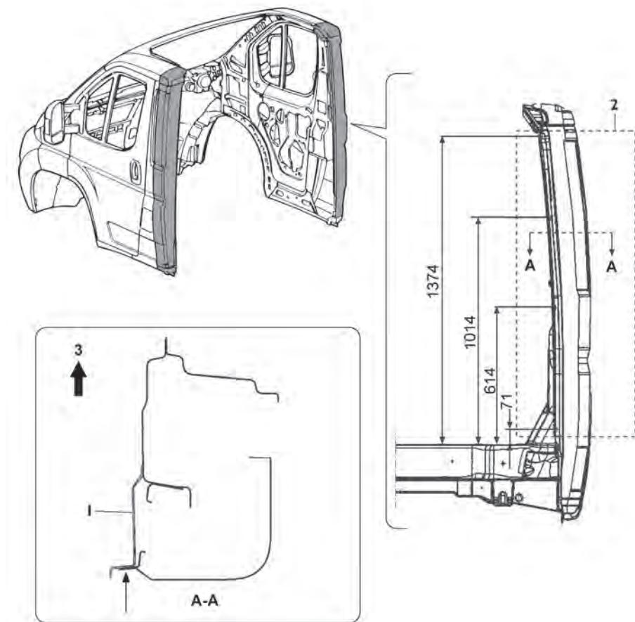
1: structural reinforcement; 2: recommended interface area; 3: direction of travel.
