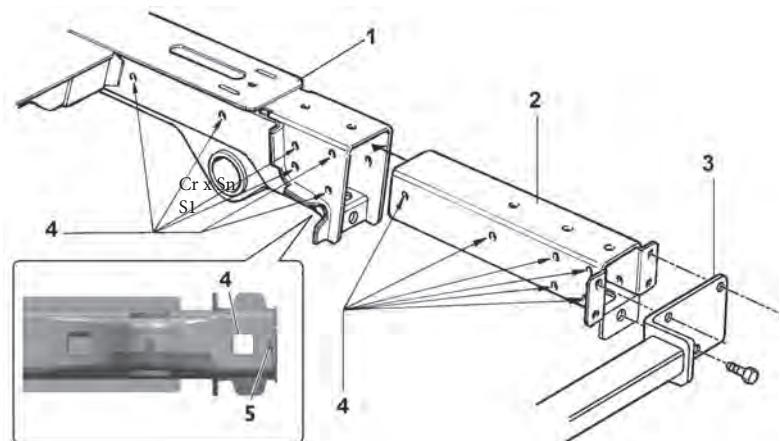
1: structure of the vehicle on which the towing hook transom bar is fastened; 2: tow hook stringer; 3: towing hook attachment flange; 4: holes for fastening assembly to chassis; 5: nut.
