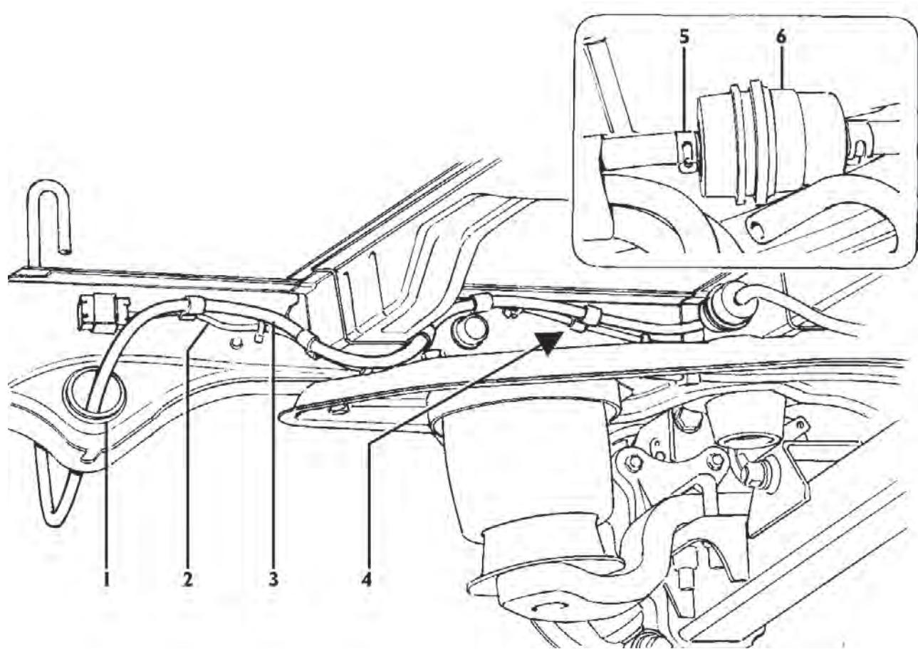
Run the pipe (3) along the left longitudinal. To fasten the rubber pipe to the corrugated sleeve of the electrical system (2) we suggest using commercially available polyamide clamps with double ring or strip (4). If you use fasteners of a different type, make sure that the cross-section of the pipe is not altered.
