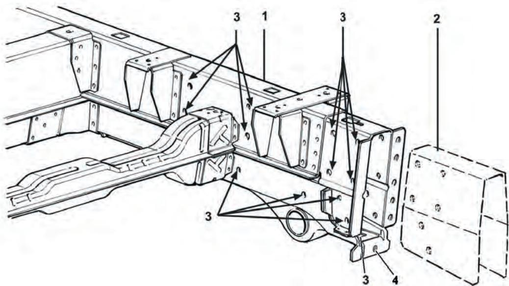
1: longitudinal member; 2: structure by coach-builder; 3: holes for fastening structure, 4: ring nut.
