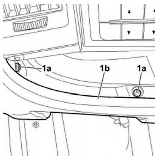
28. Put back in place the screws (1a) to fix the lower dashboard cover (1b) on the right side of the steering-wheel.
