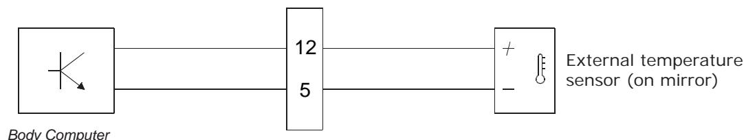
If the original New Ducato mirrors are not fitted, it is necessary to use an NTC thermistor with the following specifications:
