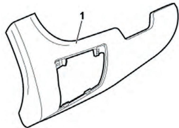
7. Undo the fixing screws (1a) for the centre pillar trim lower element (1b).
