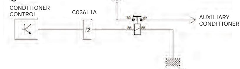
Ground point nearest to component: choice between A, B, C or pin 2 of connector C036L1C
