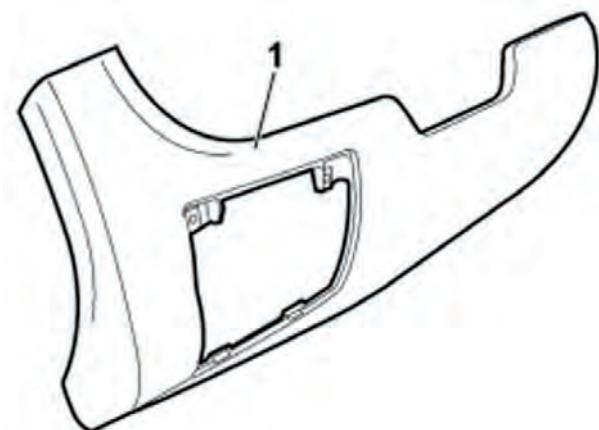
27. Put back in place the screws (1a) to fix the lower dashboard cover (1b) on the left side of the steering-wheel.
