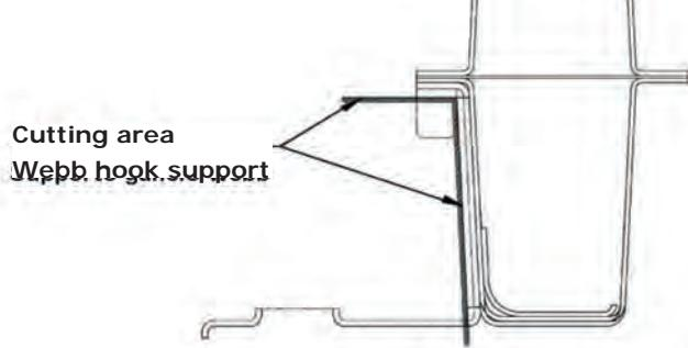
**NOTE** The mounting must be cut as shown. Restore anti-rust treatment after cutting.
