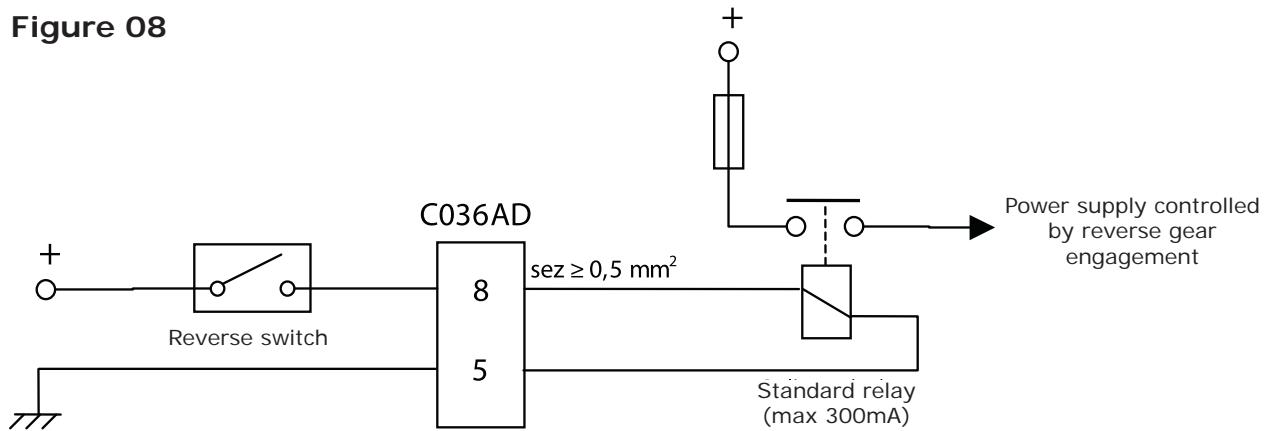
► **NOTE: When using pin 5 of connector C036AD (frame GND) for several devices ( $\Sigma I \leq 4A$ ), we recommend resorting to ultrasound welding or an equivalent equipotential connection. We strongly recommend that you do NOT use multiple crimping on the cable lugs.**
