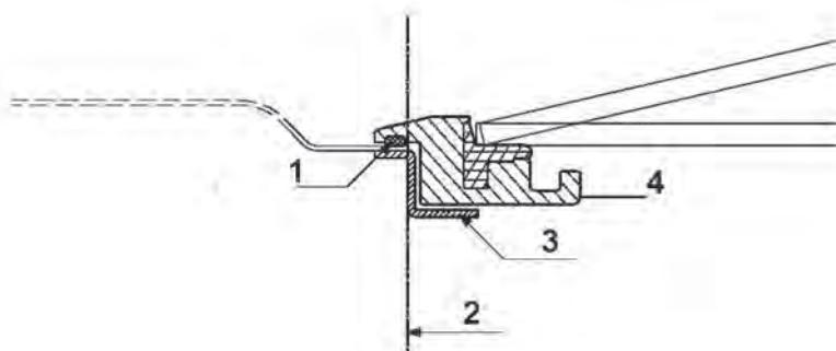
1: Sealant - 2: Cut area - 3: Attachment profile - 4. hatch
