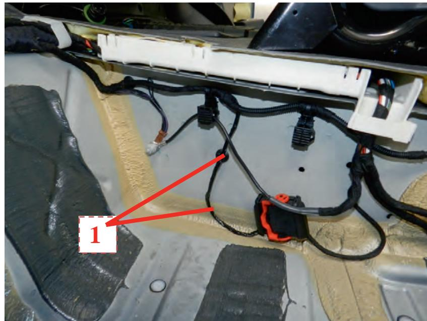
11. Thoroughly grease the rear surface of the control unit (1a) with heptane (or isopropyl alcohol) and apply a Velcro cutting (1b) of a size that ensures that the control unit remains secured.
