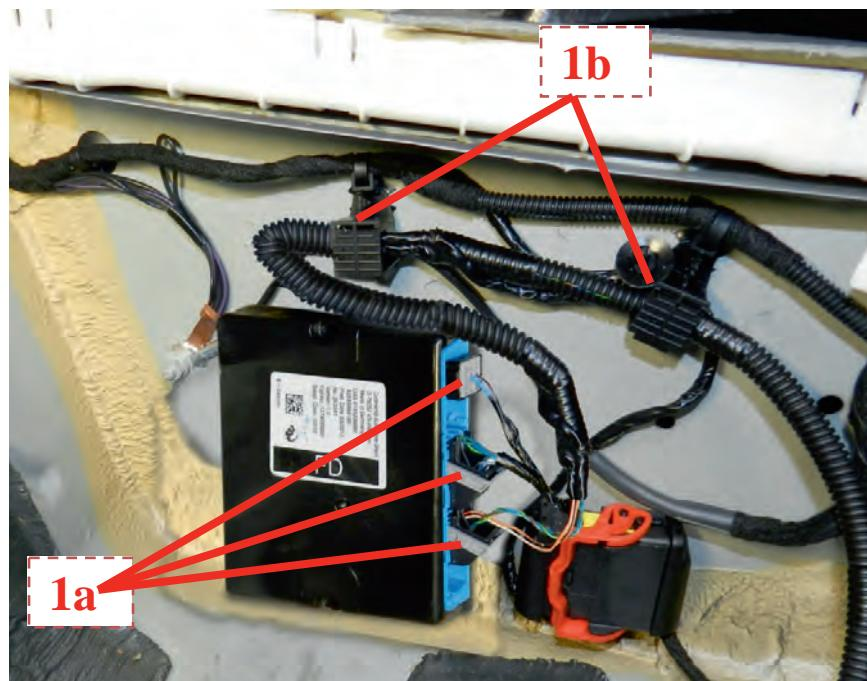
14. Place the wiring (1a) of the control unit inside the cable duct (1b) positioned on the vehicle, then secure using the clips provided.
