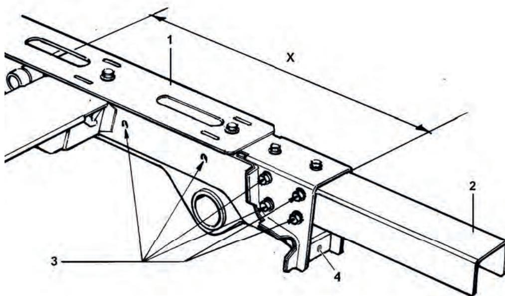
1: longitudinal member; 2: structure by coach-builder; 3: holes for fastening structure;
