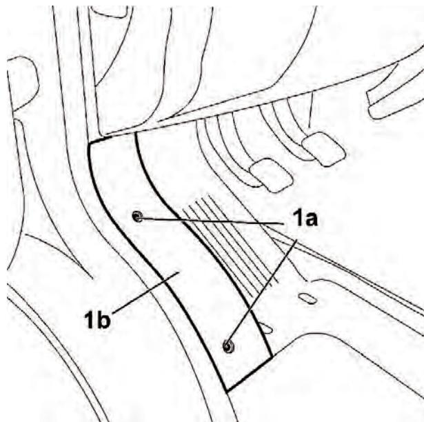
9. Undo the fixing screws (1a) and remove the kick plate (1b).
