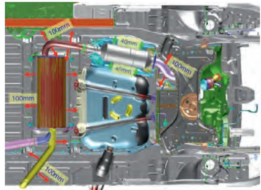
(\* ) Do NOT plan any component above the hot zone if there is no heat shield.
