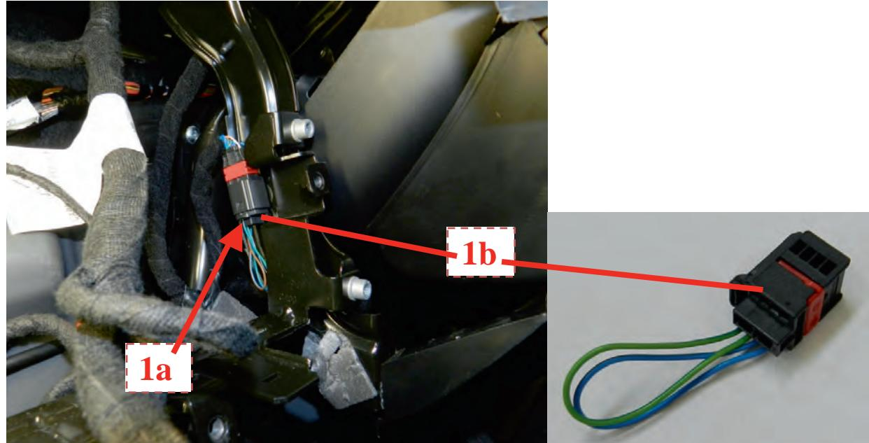
21. Connect the electrical connection of the control unit wiring, and position the wiring in the lower part of the Body Computer mounting bracket.
