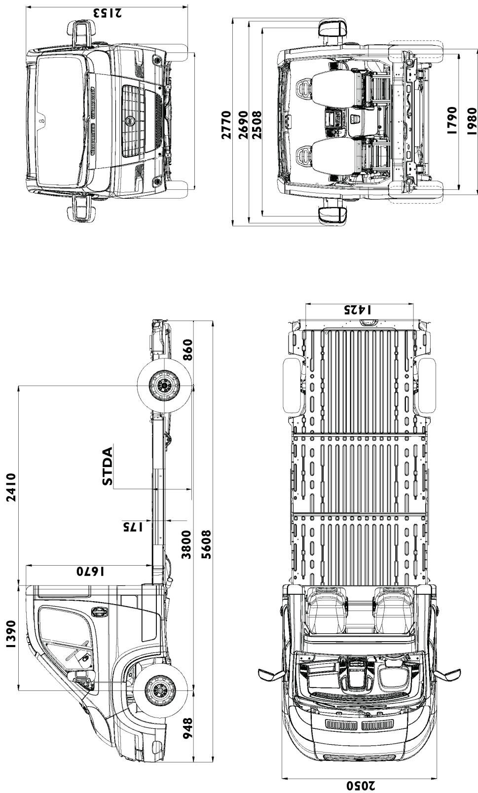
STDA: Height from ground: 550 mm (Payload 3000)
