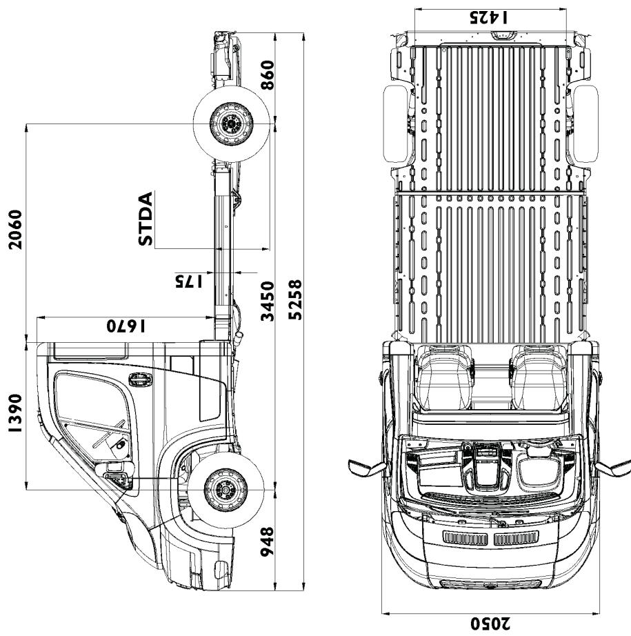
STDA: Height from ground: 545 mm (Payload 3000)
