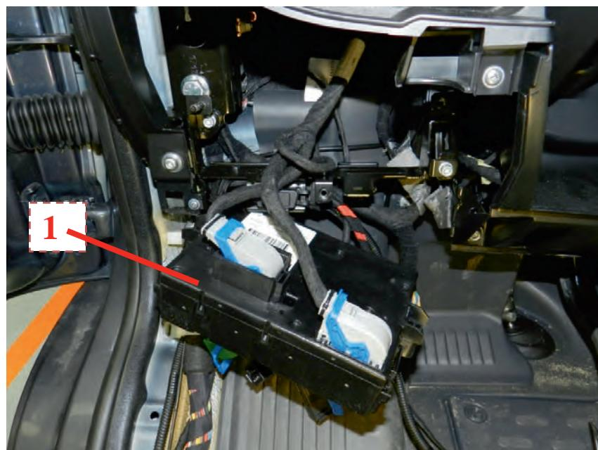
20. Press the retaining clip (1a), then disconnect and remove the short circuit connector (1b).
