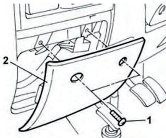
4. Undo the screw (1a) fixing the lower left trim of the dashboard (1b) located to the right of the steering wheel.
